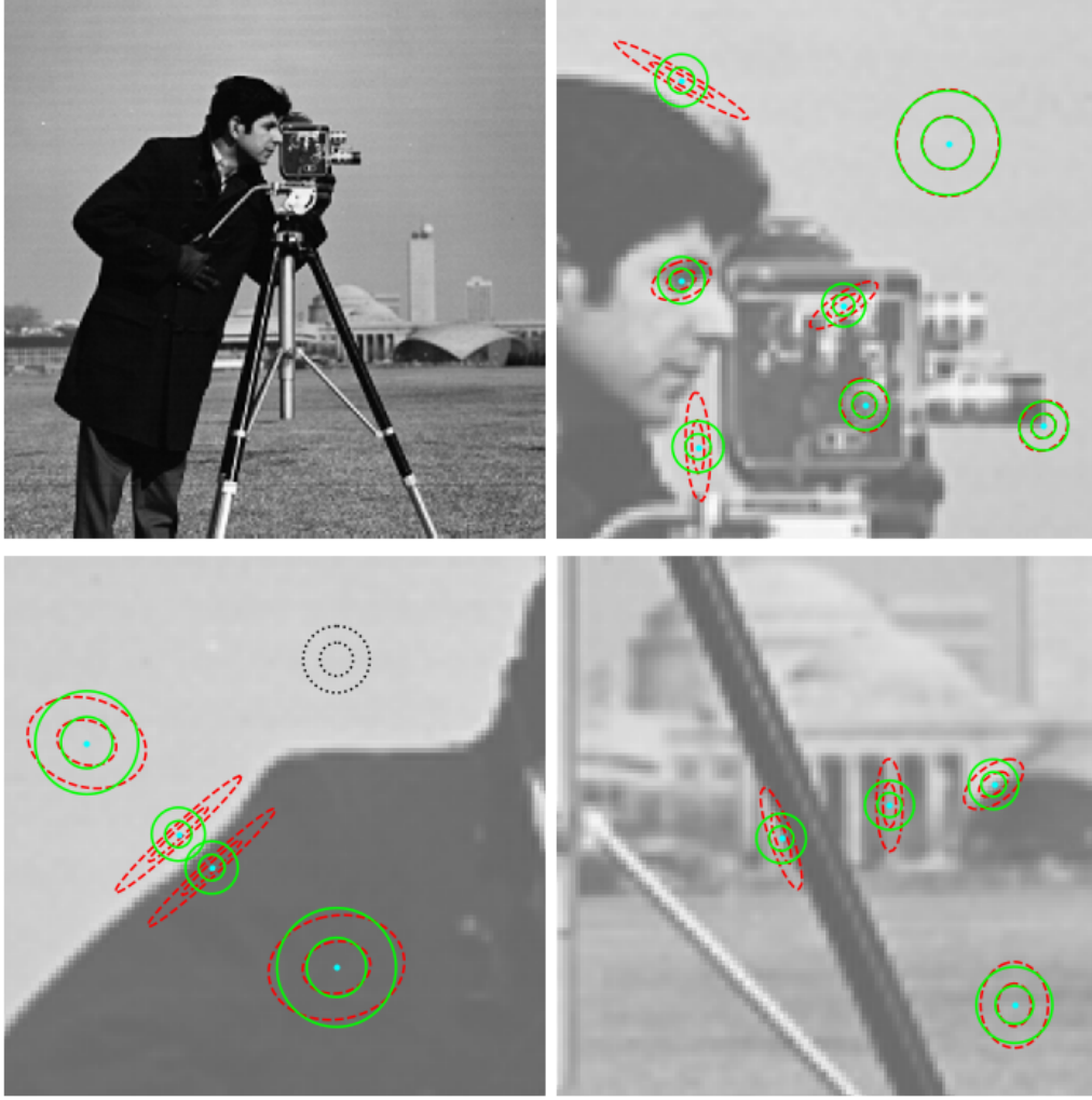
Figure 14. Comparison of the scaled (solid green) and shaped (dashed red) kernels. The upper-left image was used as an input for the test reduction where each pixel used as a sample. The bottom-left image contains a black-dotted kernel, representing the test kernel with smoothing parameter \alpha_{test} . Kernels are relatively large in smooth regions and smaller in regions containing structure. Note that the shaped kernels are stretched perpendicular to the principle gradient direction, and will preserve edges well in subsequent reductions. The data for this image was taken from skimage.data.camera (see scikitimage (2014) ).
